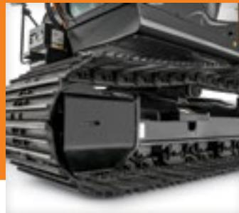
■ With large idlers, rollers and strutted track links, the sealed and lubricated undercarriage is built for the long haul.
