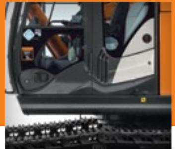
■ Reinforced D-channel side frames provide maximum cab and component protection.
