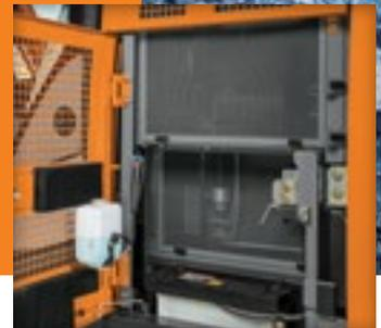
■ Ground-level-accessible coolers with easily removed pre-cleaner screens help prevent trash from plugging up the cores — helping maintain cool-running efficiency.
