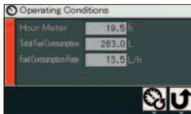
Fuel consumption per operating hour is computed, and the result is displayed on the LCD monitor. This information suggests refuelling timing, guides energy-saving operation and efficient job management.
