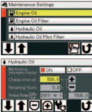
The LCD monitor provides maintenance timing alerts for the hydraulic oil and fuel filters, according to the schedule preset by the user each time the key switch is turned. Properly scheduled maintenance can prevent equipment damage and failure.
