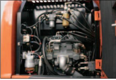
Wide doors give ground-level access to the fuel filter, water separator and engine oil filter. Hydraulic oil can be used up to 5 000 hours.
