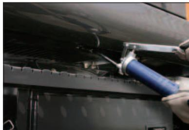
The concentrated one-spot oil refill point for swing bearing was redesigned and located underneath the cab. This results in easier greasing and maintenance.
