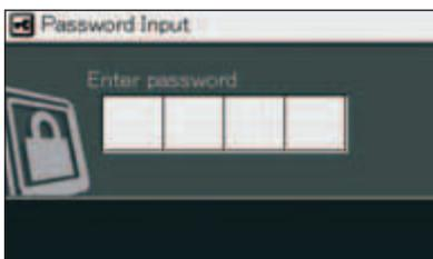
The electronic immobilizer requires the entry of an encryption code to the multifunctional monitor each time when starting the engine to prevent theft and vandalism.
